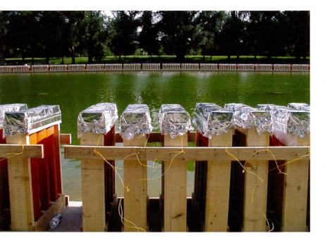
Some fireworks displays are run entirely by computers. Others need an operator to tell the firing system when to fire the shell. The operator may follow a written plan or receive instructions over a radio. When the operator presses a button on the equipment, it sends an electrical signal through a lat to one of the electric matches. This creates a spark that ignites the shell's fuse, creates an explosion, and launches the firework into the air.
